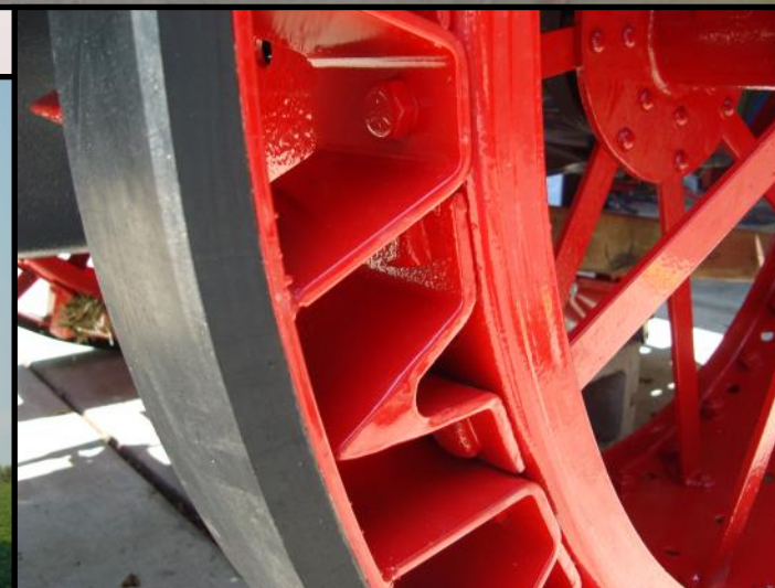
Had steel offset bands fabricated then covered in thick rubber to smooth out the ride but retain the original wheel and look.
