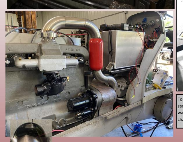
lests helped us to hind problem areas prior to first startup. We found 2 issues after startup that could have resulted in catastrophic failure but close eye on oiling saved us. One original internal oil plug failed but was caught in time.
