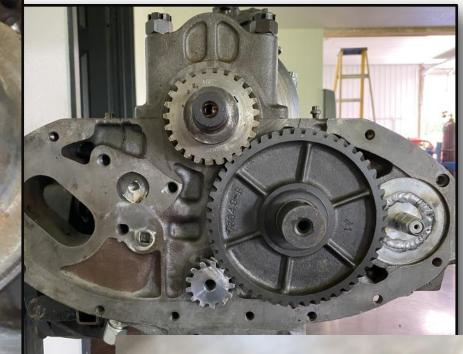
A custom gear was locally manufactured to allow the engine to have a working governor. Many hours went into building a custom governor mechanism.
