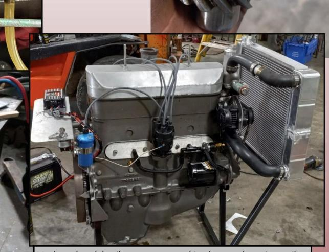
Much work and detail to get a part machined to match a spin on oil filter to the original block. Aluminum side plates allow for external oil lines to spray the cam and lower end. A custom starter (gm starter with Ford 5.4 ring gear) & water pump were also fabricated.
