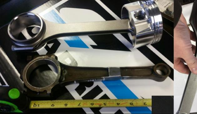
A hand fabricated rod was constructed and sent off to Carrillo who designed & machined amazing one of kind billet piston/rod combo. Corvette style pistons with Ford 460 rod journals. Works of Art!
